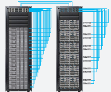
Cisco UCS is wired with a single redundant network to support all I/O
